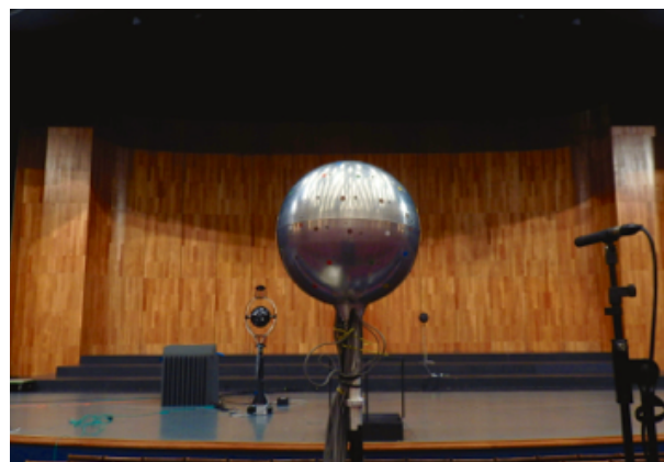
Acoustic measures at Grosses Festspielhaus in Salzburg combining a spherical microphone array (64 capsules) developed at IRCAM and a spherical loudspeakers array developed at RWTH (Aachen). Photo © Olivier Warusfel
