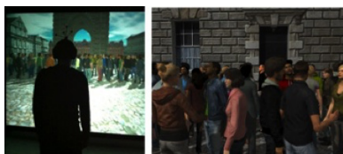
VR system in IRCAM's studio 4. The visual stereo is projected on a large screen. Visual and auditory information is updated using a position-following system.
