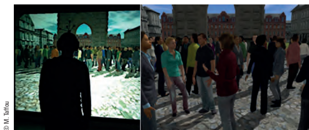
VR device in IRCAM's studio 4. Visual stereo is projected on a large screen. The visual and auditory information is updated by a position tracking system.
